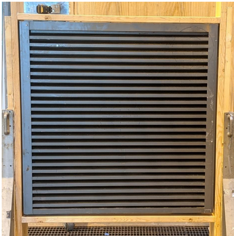
Photo No. 1 4" Rain-Resistant, Horizontal Louver Prior to Testing
